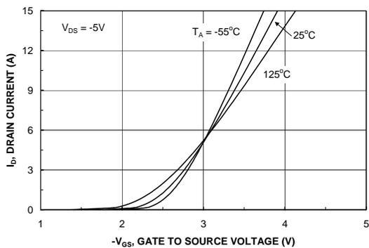
Figure 5. Transfer Characteristics.
