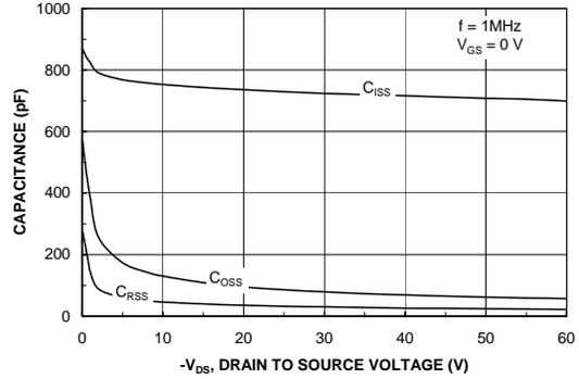
Figure 8. Capacitance Characteristics.
