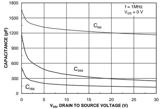
Figure 8. Capacitance Characteristics
