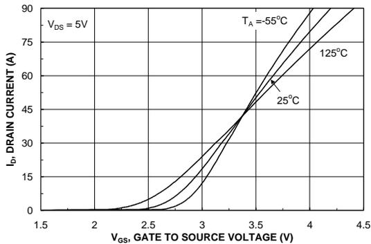
**Figure 5. Transfer Characteristics**
