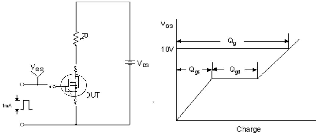
**Resistive Switching Test Circuit & Waveforms**
