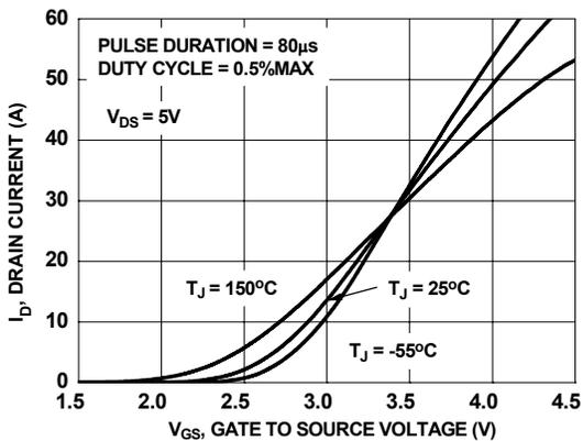
**Figure 5. Transfer Characteristics**
