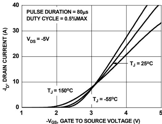
**Figure 18. Transfer Characteristics**
