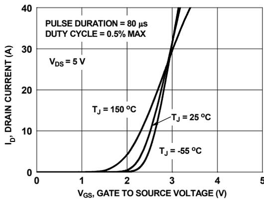
**Figure 5. Transfer Characteristics**
