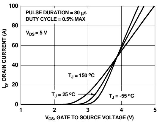
Figure 5. Transfer Characteristics
