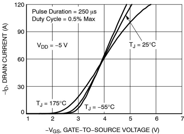
Figure 7. Transfer Characteristics
