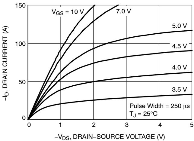
Figure 9. Saturation Characteristics
