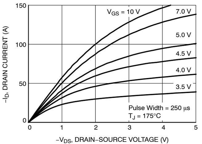
Figure 10. Saturation Characteristics
