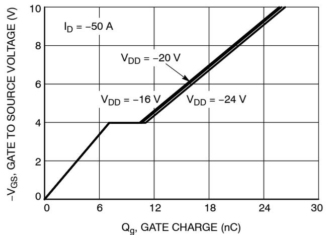
Figure 16. Gate Charge vs. Gate to Source Voltage
