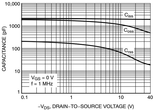
Figure 15. Capacitance vs. Drain to Source Voltage
