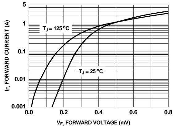
**Figure 12. Schottky Diode Forward Voltage**
