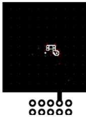
c. 110 °C/W when mounted on a 1 in<sup>2</sup> pad of 2 oz copper.
