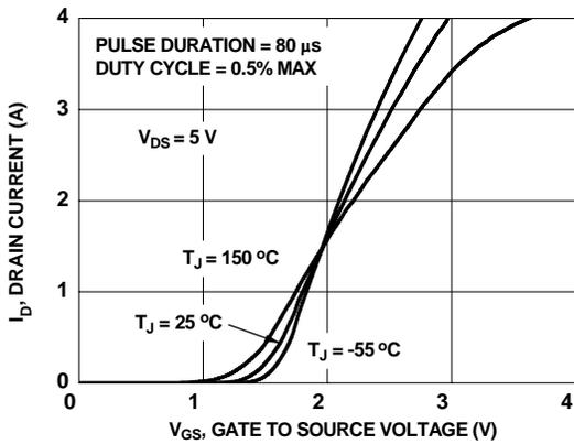
Figure 5. Transfer Characteristics
