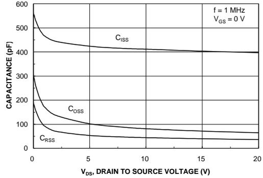
Figure 8. Capacitance Characteristics.
