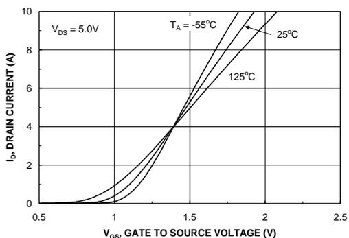
Figure 5. Transfer Characteristics.
