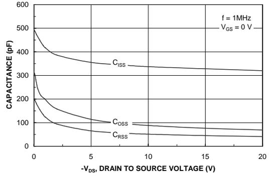
Figure 8. Capacitance Characteristics.
