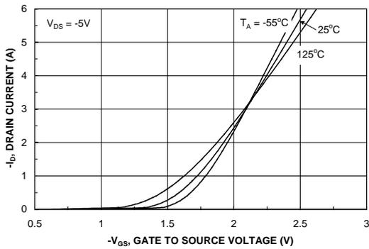
Figure 5. Transfer Characteristics.
