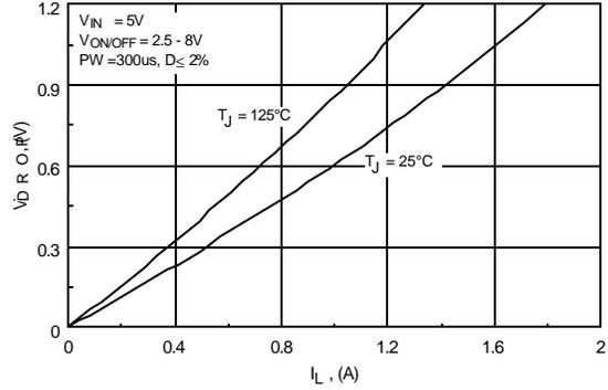
**Figure 2. Conduction Voltage Drop Variation with Load Current.**
