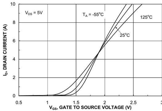
Figure 5. Transfer Characteristics.
