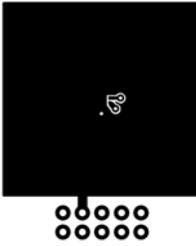
a.  $86\text{ }^\circ\text{C/W}$  when mounted on a 1 in<sup>2</sup> pad of 2 oz copper
