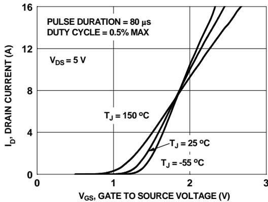
**Figure 5. Transfer Characteristics**
