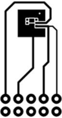
e.  $160\text{ }^\circ\text{C/W}$  when mounted on 30mm<sup>2</sup> pad of 2 oz copper
