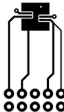
f.  $133\text{ }^\circ\text{C/W}$  when mounted on 30mm<sup>2</sup> of 2 oz copper
