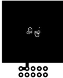
c.  $69\text{ }^\circ\text{C/W}$  when mounted on a 1 in<sup>2</sup> pad of 2 oz copper
