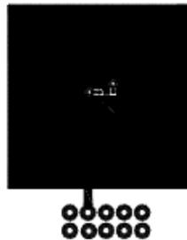
a. 52  $^\circ\text{C/W}$  when mounted on a 1 in<sup>2</sup> pad of 2 oz copper.
