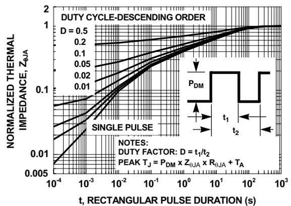
Figure 12. Transient Thermal Response Curve
