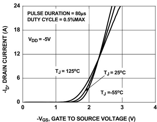
**Figure 5. Transfer Characteristics**
