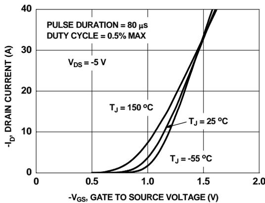
**Figure 5. Transfer Characteristics**
