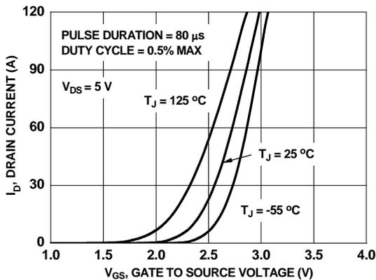
**Figure 5. Transfer Characteristics**
