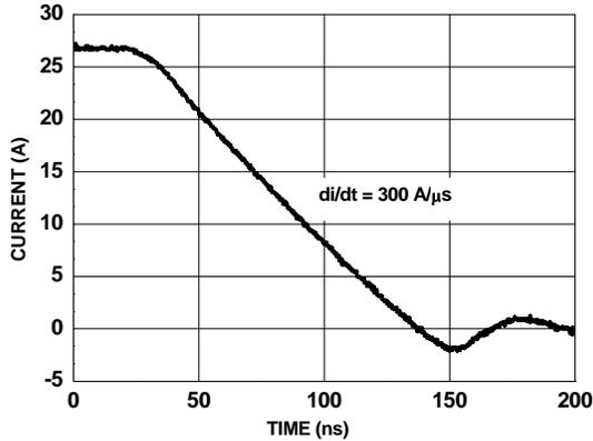
Figure 14. FDMC2512SDC SyncFET body diode reverse recovery characteristic
