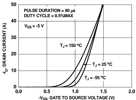
**Figure 5. Transfer Characteristics**
