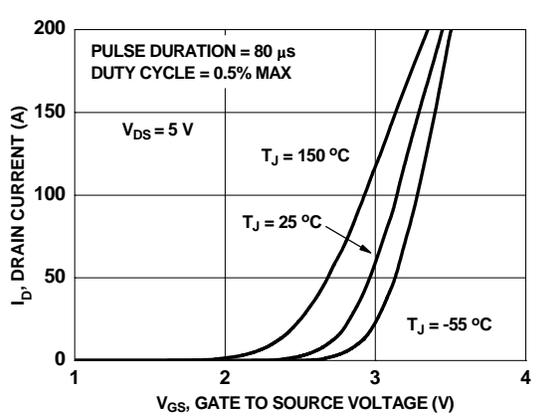
Figure 5. Transfer Characteristics
