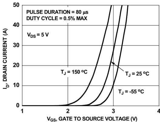
**Figure 5. Transfer Characteristics**
