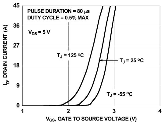
Figure 5. Transfer Characteristics
