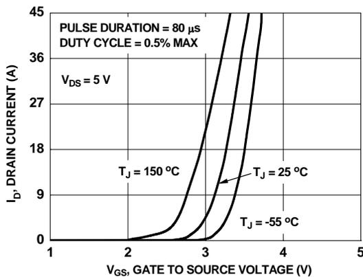
Figure 5. Transfer Characteristics
