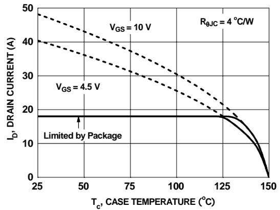
**Figure 22. Maximum Continuous Drain Current vs Case Temperature**
