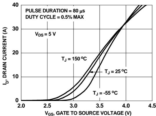
**Figure 5. Transfer Characteristics**
