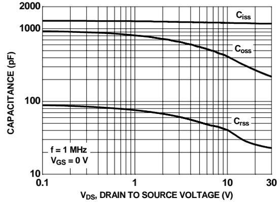
**Figure 20. Capacitance vs Drain to Source Voltage**
