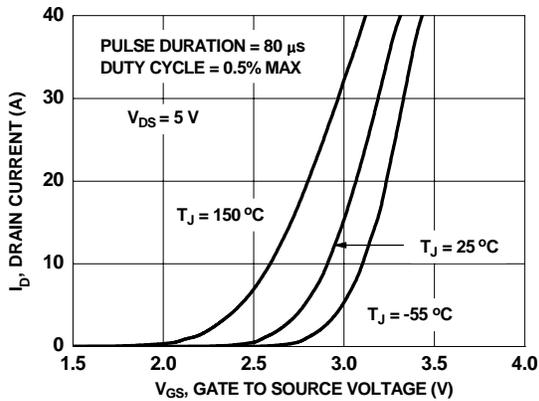
Figure 17. Transfer Characteristics
