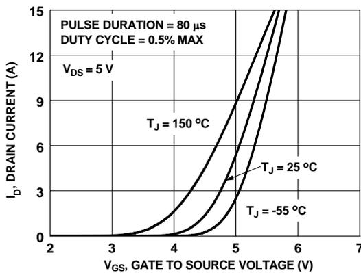
Figure 5. Transfer Characteristics
