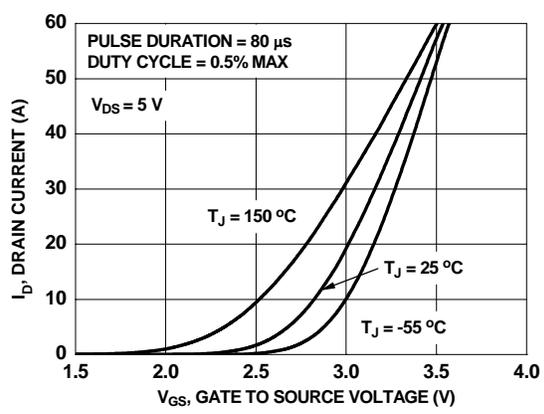
Figure 5. Transfer Characteristics
