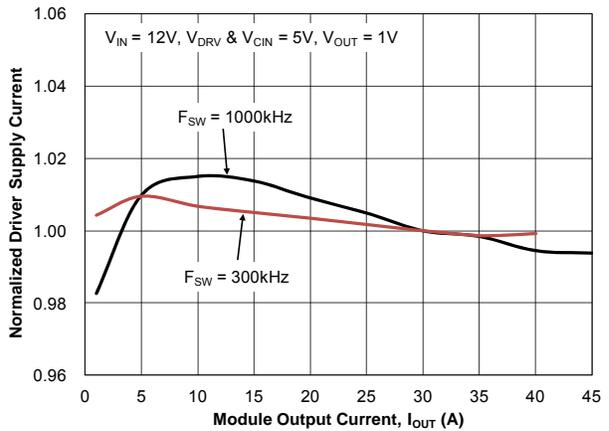
Figure 17. Driver Supply Current vs. Output Current
