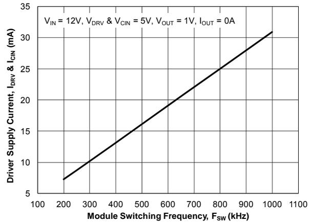
Figure 15. Driver Supply Current vs. Switching Frequency
