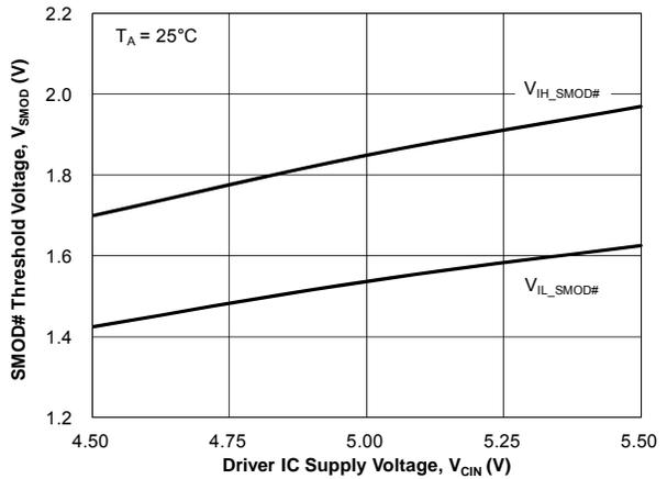
Figure 21. SMOD# Threshold vs. Driver Supply Voltage
