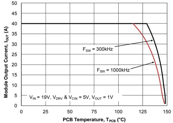
Figure 7. Safe Operating Area for 19V<sub>IN</sub>
