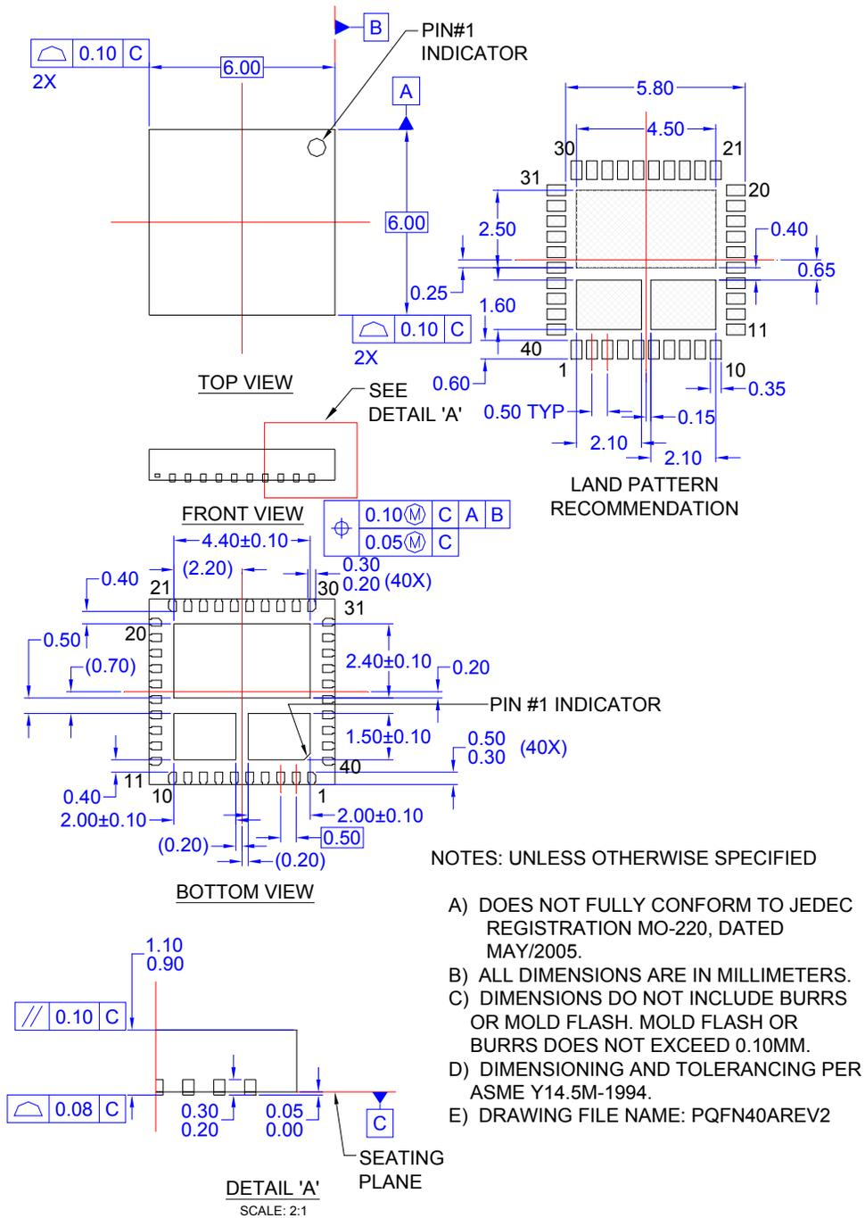
**Figure 35. 40-Lead, Clipbond PQFN DrMOS, 6.0x6.0mm Package**
