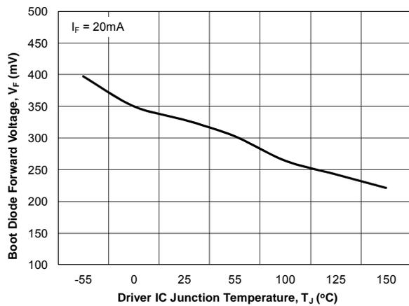
**Figure 27. Boot Diode Forward Voltage vs. Temperature**
