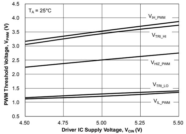
Figure 19. PWM Threshold vs. Driver Supply Voltage
