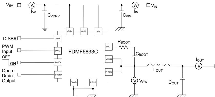
Figure 32. Power Loss Measurement
