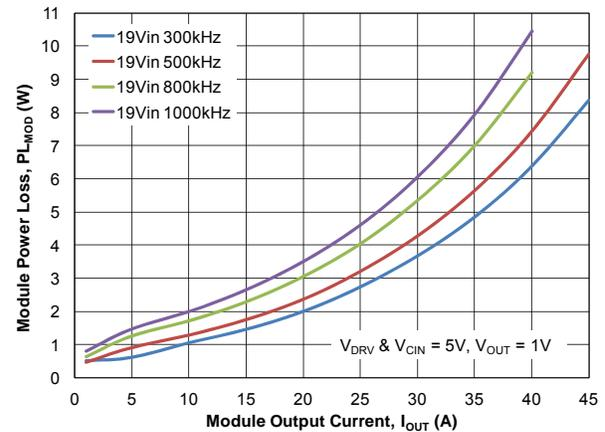
Figure 9. Power Loss vs. Output Current for 19V<sub>IN</sub>
