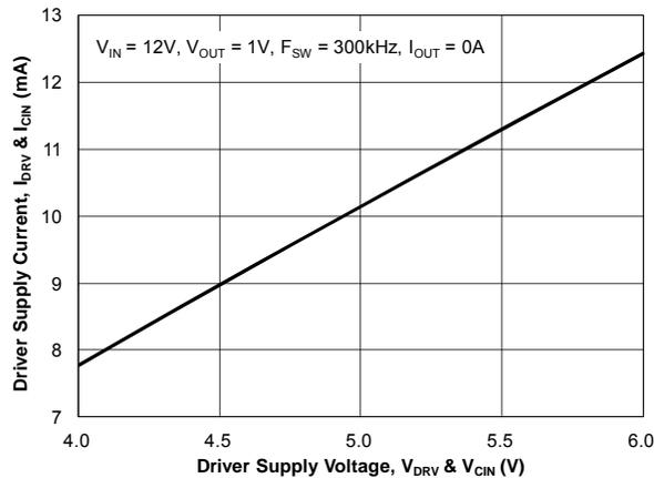
Figure 16. Driver Supply Current vs. Driver Supply Voltage
