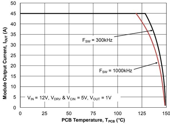
Figure 6. Safe Operating Area for 12V<sub>IN</sub>
