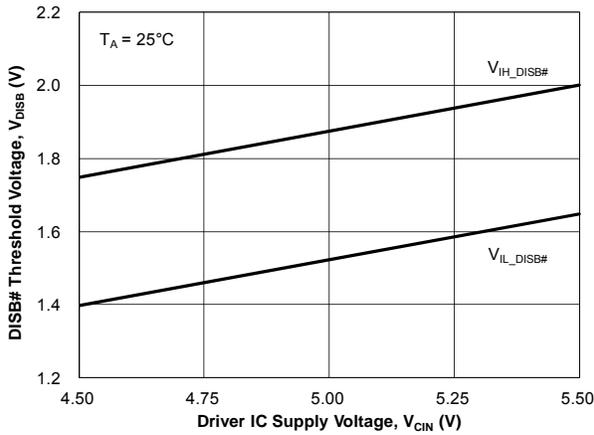
**Figure 24. DISB# Threshold vs. Driver Supply Voltage**
