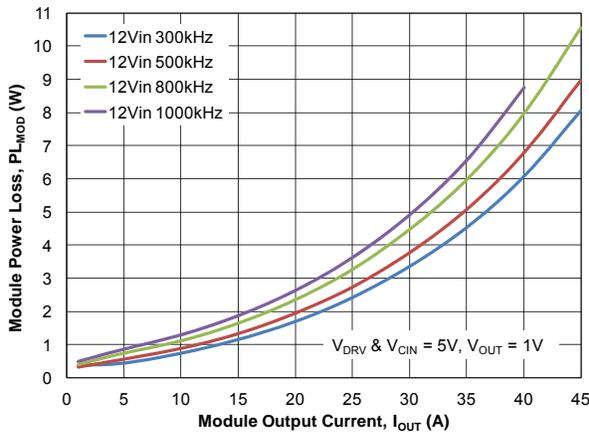
Figure 8. Power Loss vs. Output Current for 12V<sub>IN</sub>
