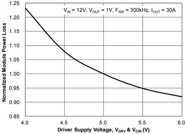
Figure 12. Power Loss vs. Driver Supply Voltage
