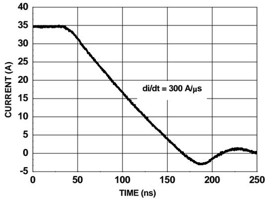
Figure 14. FDMS2502SDC SyncFET body diode reverse recovery characteristic
