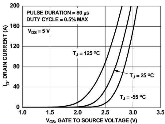
**Figure 5. Transfer Characteristics**
