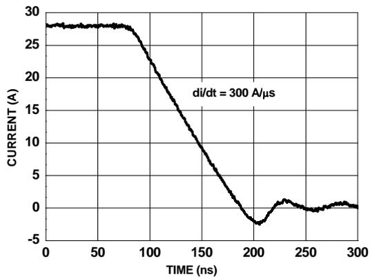
Figure 14. FDMS3008SDC SyncFET body diode reverse recovery characteristic
