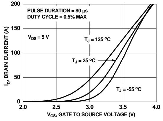
Figure 5. Transfer Characteristics
