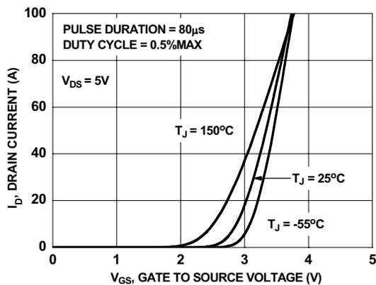
Figure 5. Transfer Characteristics
