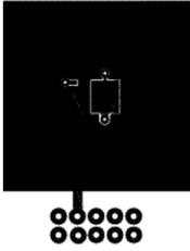
a. 57 °C/W when mounted on a 1 in<sup>2</sup> pad of 2 oz copper
