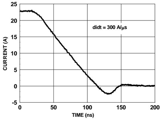
Figure 27. FDMS3604AS SyncFET body diode reverse recovery characteristic
