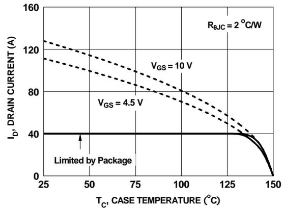
**Figure 23. Maximum Continuous Drain Current vs Case Temperature**
