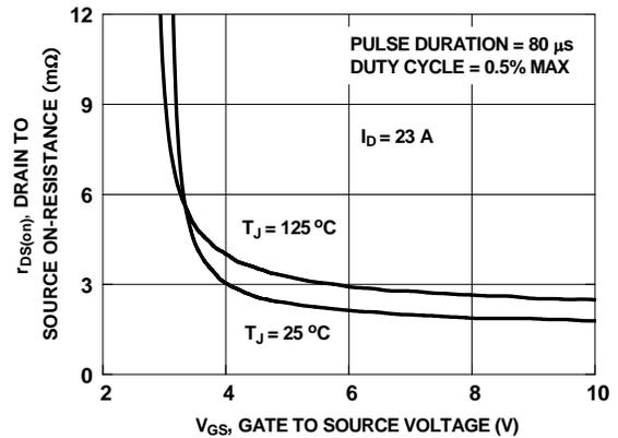
Figure 17. On-Resistance vs Gate to Source Voltage
