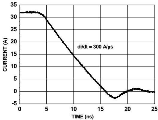
Figure 14. FDMS7558S SyncFET body diode reverse recovery characteristic
