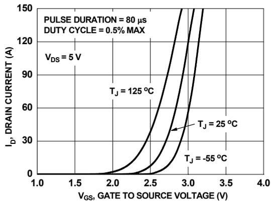
Figure 5. Transfer Characteristics
