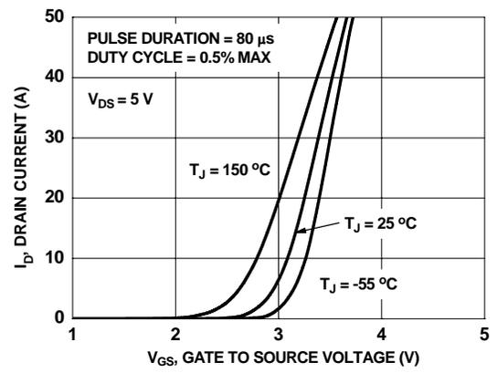
**Figure 5. Transfer Characteristics**
