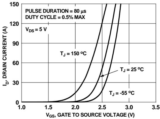
Figure 5. Transfer Characteristics
