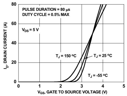
**Figure 5. Transfer Characteristics**
