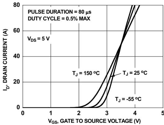
**Figure 5. Transfer Characteristics**
