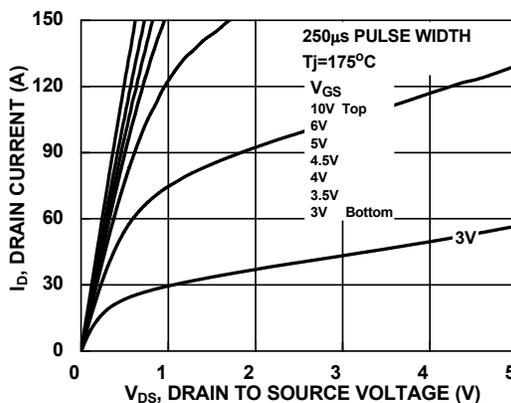
Figure 10. Saturation Characteristics
