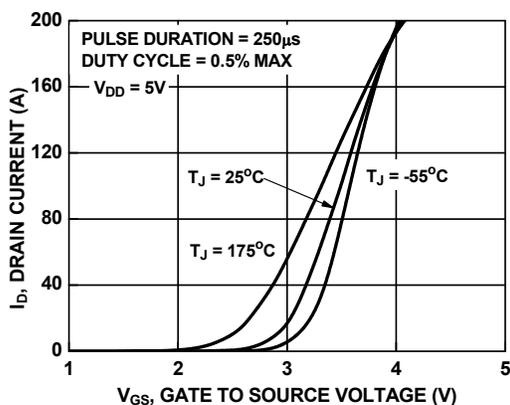
Figure 7. Transfer Characteristics
