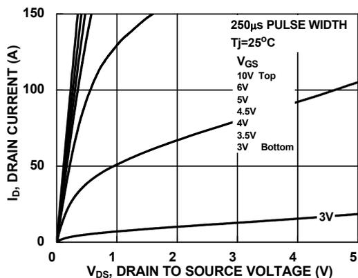
Figure 9. Saturation Characteristics
