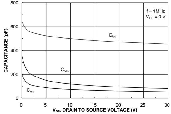
Figure 8. Capacitance Characteristics.
