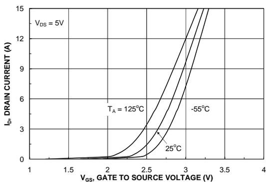
Figure 5. Transfer Characteristics.
