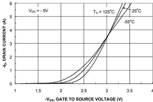
**Figure 5. Transfer Characteristics.**
