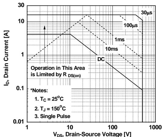
**Figure 9. Maximum Drain Current**
