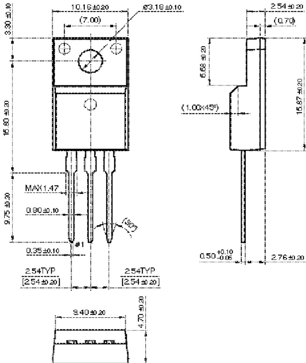
\* Front/Back Side Isolation Voltage : AC 2500V
