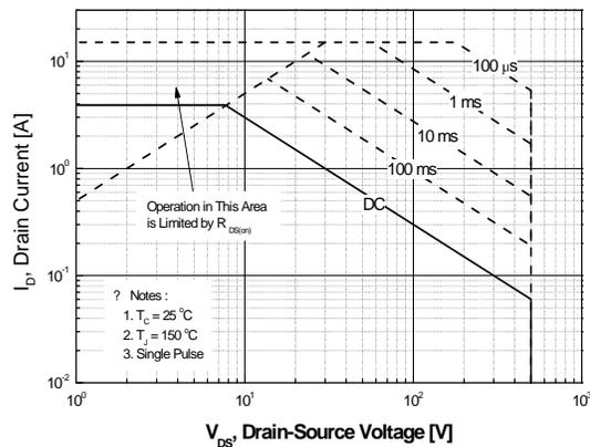
**Figure 9. Maximum Drain Current**
