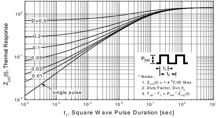
**Figure 10-2. Transient Thermal Response Curve - FDPF7N50U**
