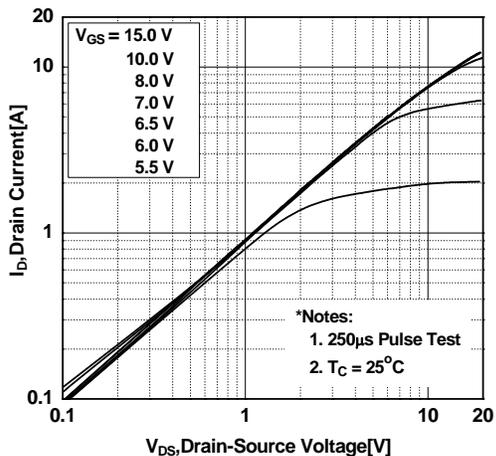
**Figure 2. Transfer Characteristics**
