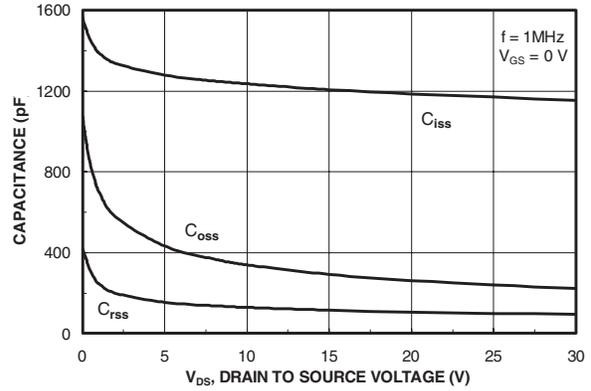
**Figure 8. Capacitance Characteristics.**
