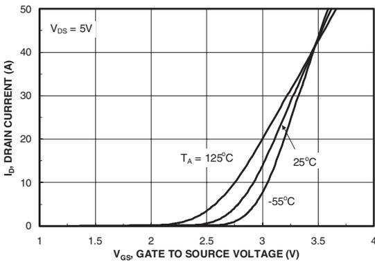
Figure 5. Transfer Characteristics.
