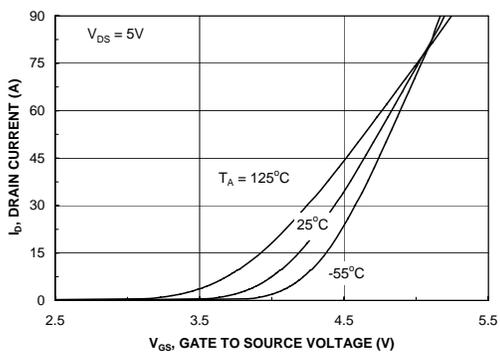
Figure 5. Transfer Characteristics.
