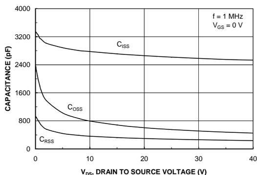
Figure 8. Capacitance Characteristics.
