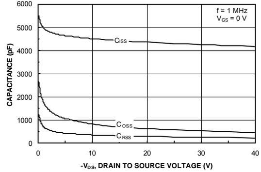
Figure 8. Capacitance Characteristics.
