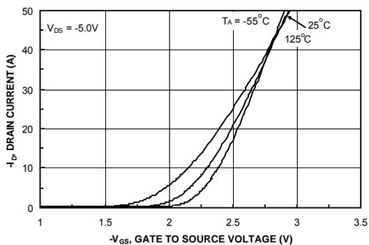
Figure 5. Transfer Characteristics.
