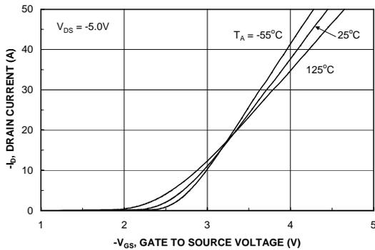
Figure 5. Transfer Characteristics.
