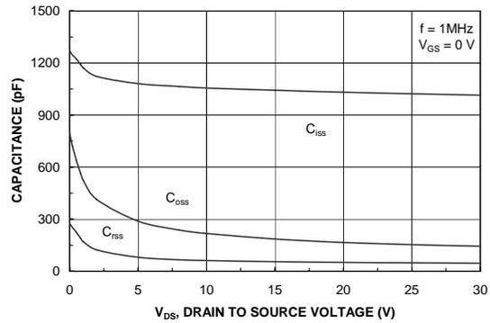
Figure 8. Capacitance Characteristics.
