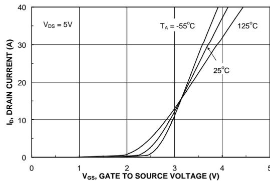
Figure 5. Transfer Characteristics.
