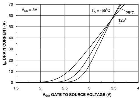
Figure 5. Transfer Characteristics.
