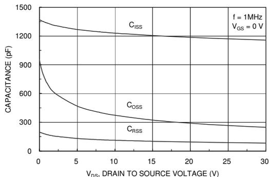
Figure 8. Capacitance Characteristics.
