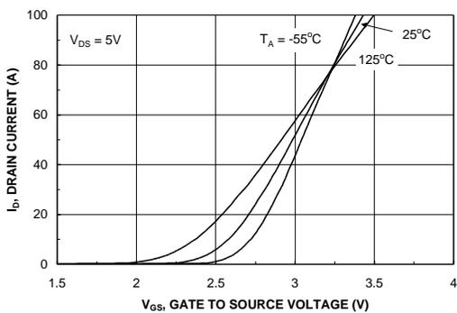
Figure 5. Transfer Characteristics.
