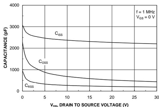
Figure 8. Capacitance Characteristics.
